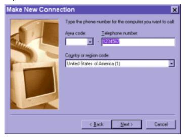
After clicking on \_\_\_\_\_\_, this new connection will display in the Dial-up Networking folder and will be used for null modem connections.
